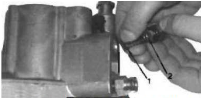
Fig 3 Installing spring and discharge fitting
