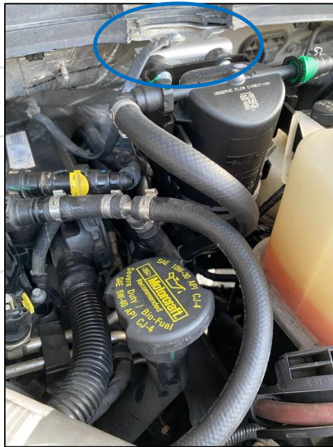
Figure 4: Bracket mounted, filter installed, hoses attached
