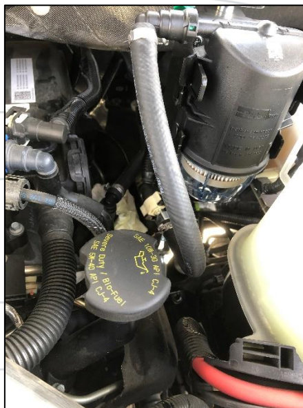
Figure 11: Proper Hose Clearance
