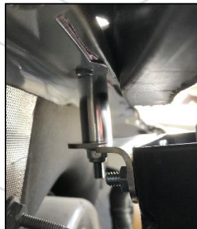
Figure 7: Bracket installed with spacer
