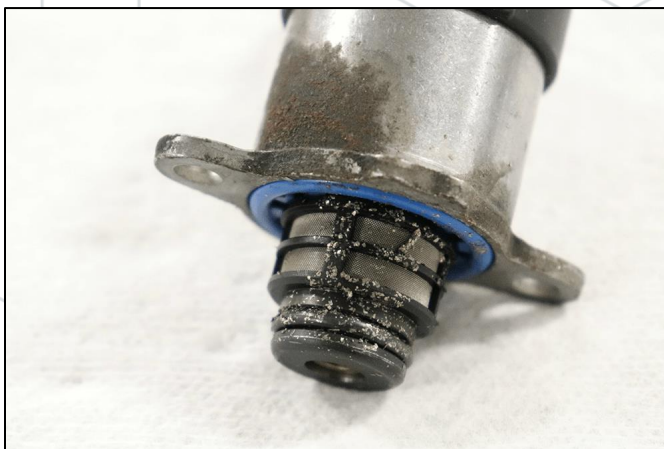
Figure 7: Failing CP4 FCA
