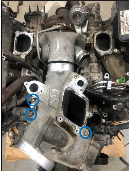
Figure 5: Lower Intake Bolts
