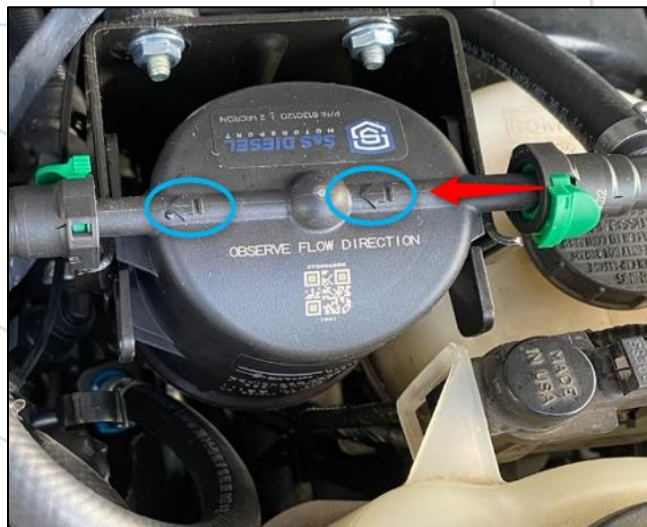
Figure 5: Filter orientation and flow direction
